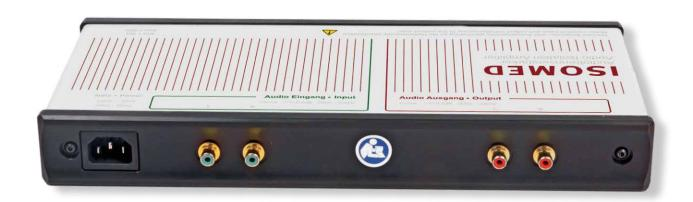
Two audio signals can be connected via the green cinch input channels. The red cinch sockets deliver the galvanically isolated output signals.
